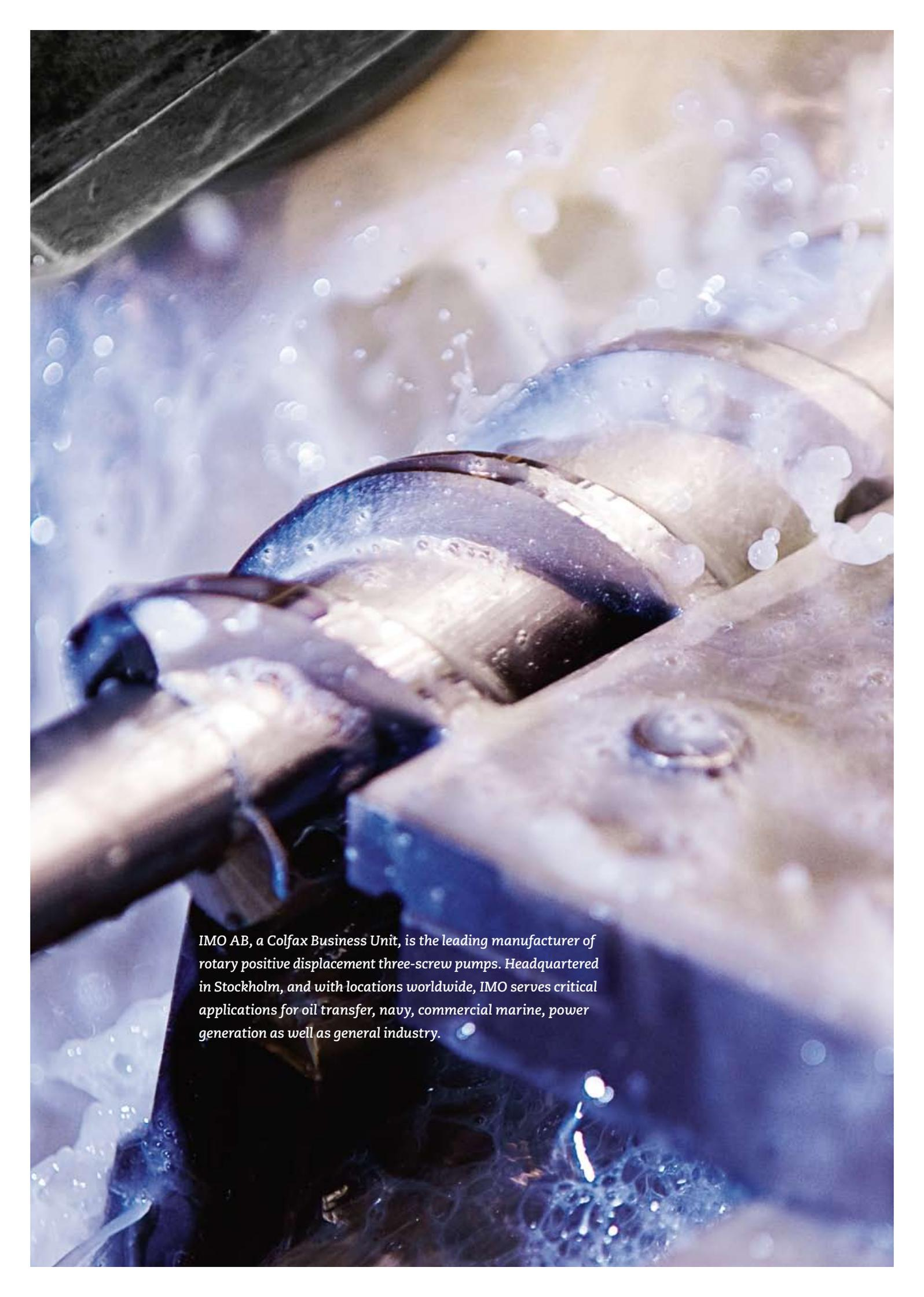
A close-up, high-angle photograph of a three-screw pump mechanism. The central screw is the focal point, surrounded by two other screws. The entire assembly is encased in a metal housing. Water is splashing around the mechanism, creating a dynamic and industrial atmosphere. The lighting is dramatic, with strong highlights and deep shadows, emphasizing the metallic textures and the motion of the water.
